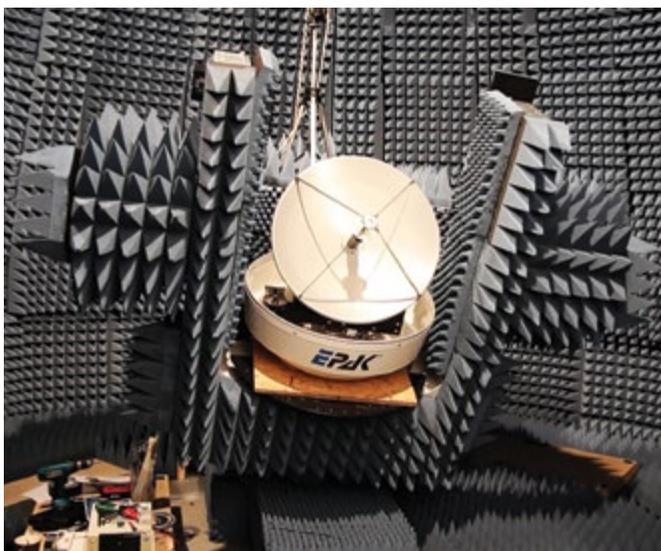
**Figure 2: The DSi6 antenna from EPAK while being tested at the Fraunhofer Facility for Over-the-air Research and Testing (FORTE)**
