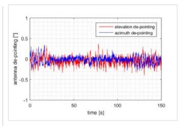
Figure 3: De-pointing estimation results of the DSi6 antenna from EPAK when tested on the maritime Class A standard motion profile developed by Fraunhofer IIS
