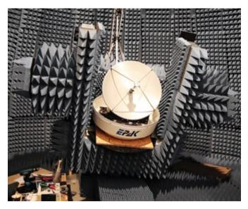
Figure 2: The DSi6 antenna from EPAK while being tested at the Fraunhofer Facility for Over-the-air Research and Testing (FORTE)
