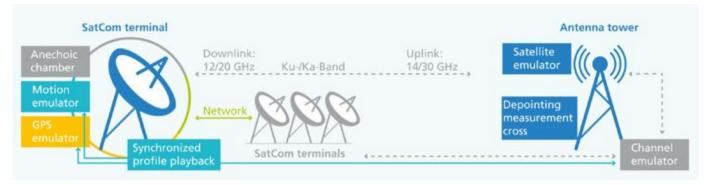
Figure 1: An overview of the structure of the Fraunhofer Facility for over-the-air Research and Testing (FORTE)
