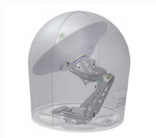
Technical Drawing of EPAK DS13, maritime VSAT antenna with 130 cm reflector diameter in protective dome
